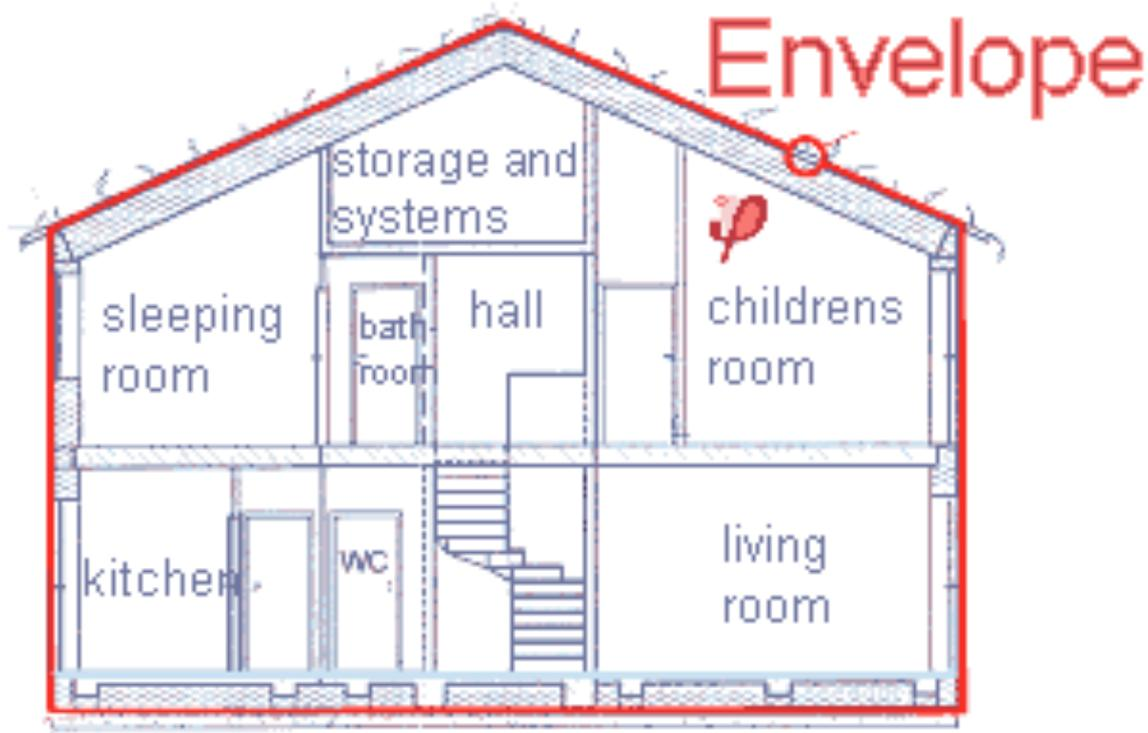
It is convenient, to define the envelope for energy balances of a building at the external surface of the insulation.
