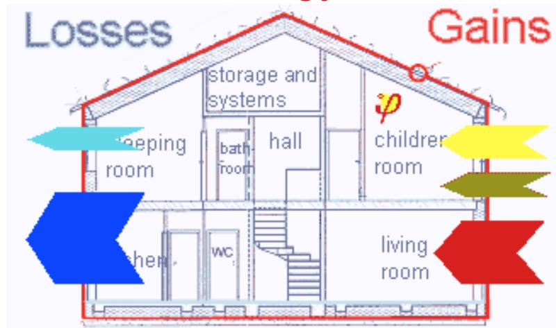
**Free “heat gains”**: e.g. solar radiation entering through windows (**passive solar energy**) and the energy which enters the house through the electricity supply and is converted to the so-called **“internal heat sources”**
