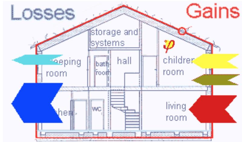
**“Heating” therefore, is only a replacement of this heat loss and can therefore be reduced by more effective prevention of losses.**
